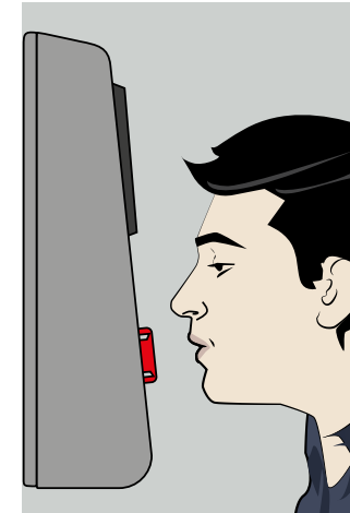
Passive test with an Alcolizer Centurion Zero Tolerance instrument
